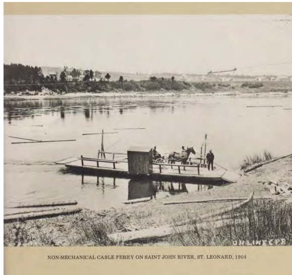
Non mechanical Ferry on the Saint John River. St. Leonard 1904. The person pulled on the rope, to move the ferry across the river.
