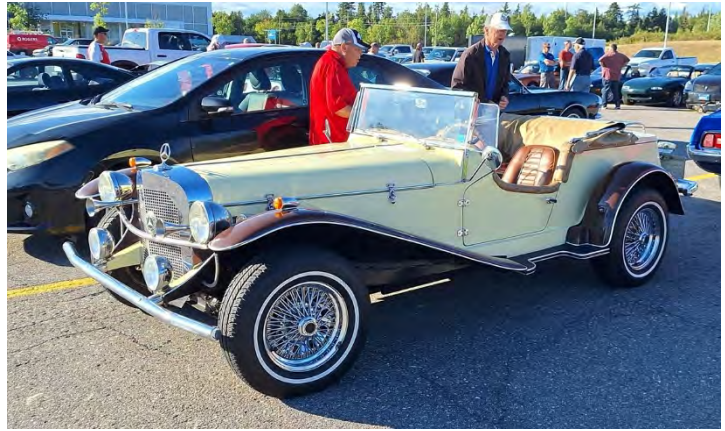
This is a 1929 Mercedes KIT car. Frame is a Ford and the body is a kit component made of fiberglass.
